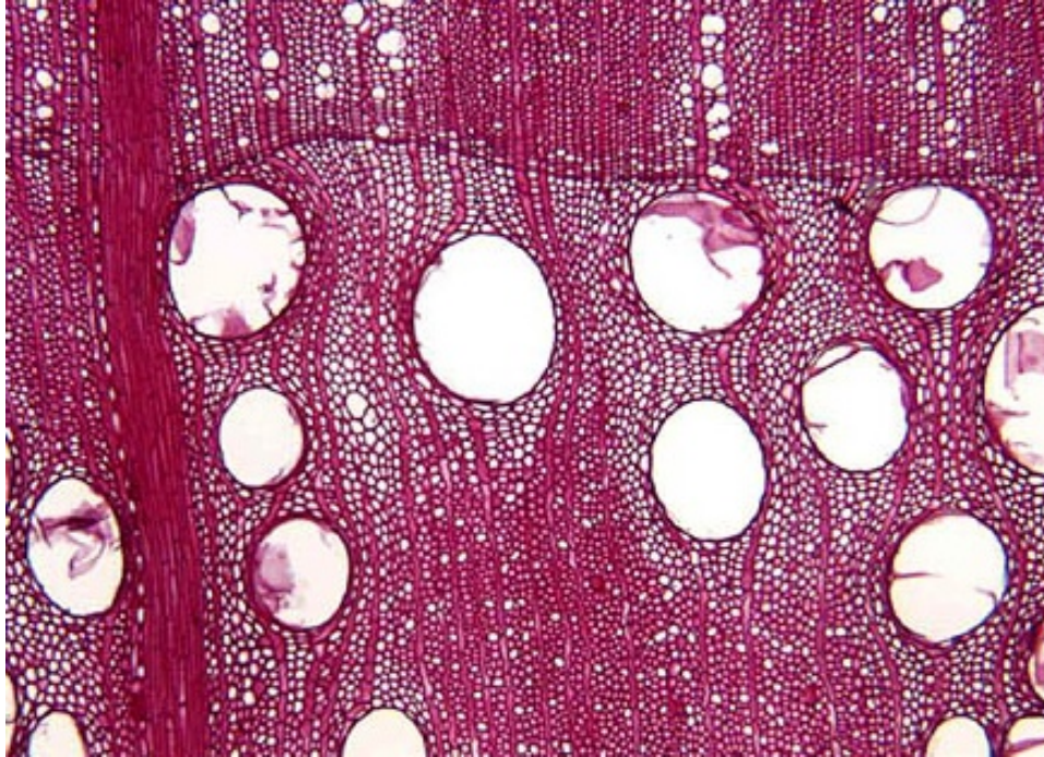
Transverse section of wood from white oak.
